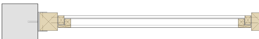
Fig. 45 – Junction with a C shaped steel element between reinforced concrete column and timber post, and timber panel section, with a primary fixed frame and a secondary opening frame.
