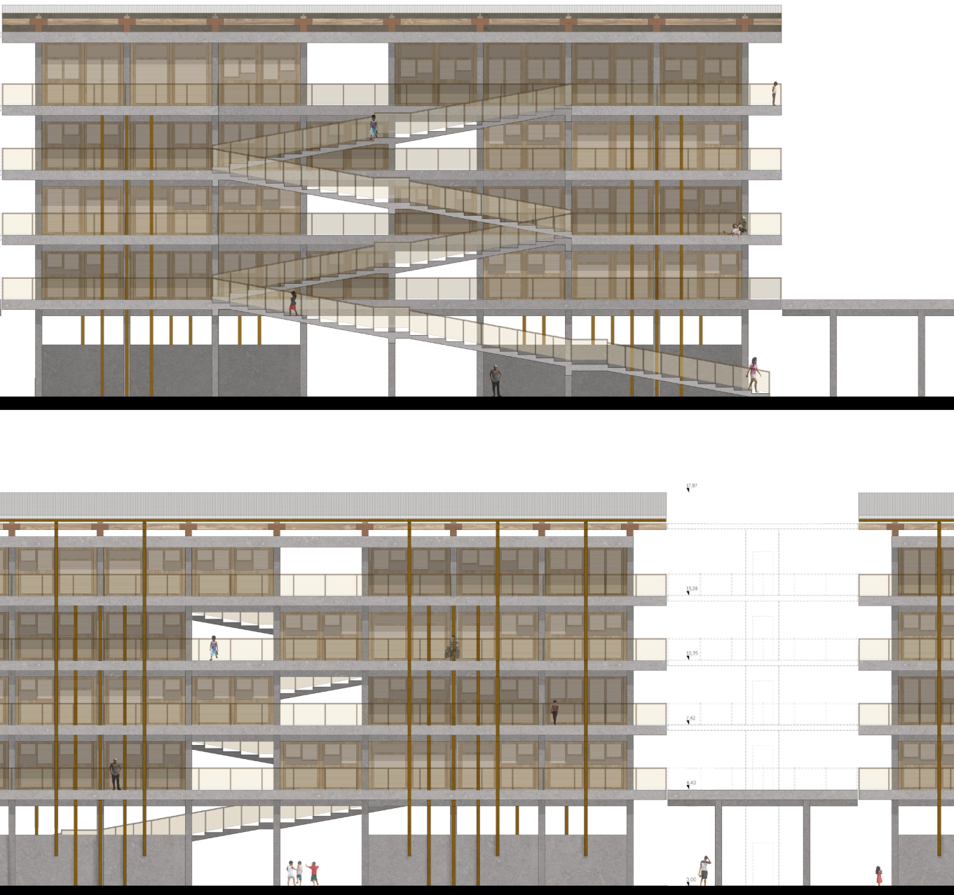
Fig. 42 – (from the top) Elevation on the street side, transversal section and elevation along S.M. side. All the vertical elements follow modules and sub-modules of the structural system, interrupting, together with the stairwell, the prominent horizontality of the building.
