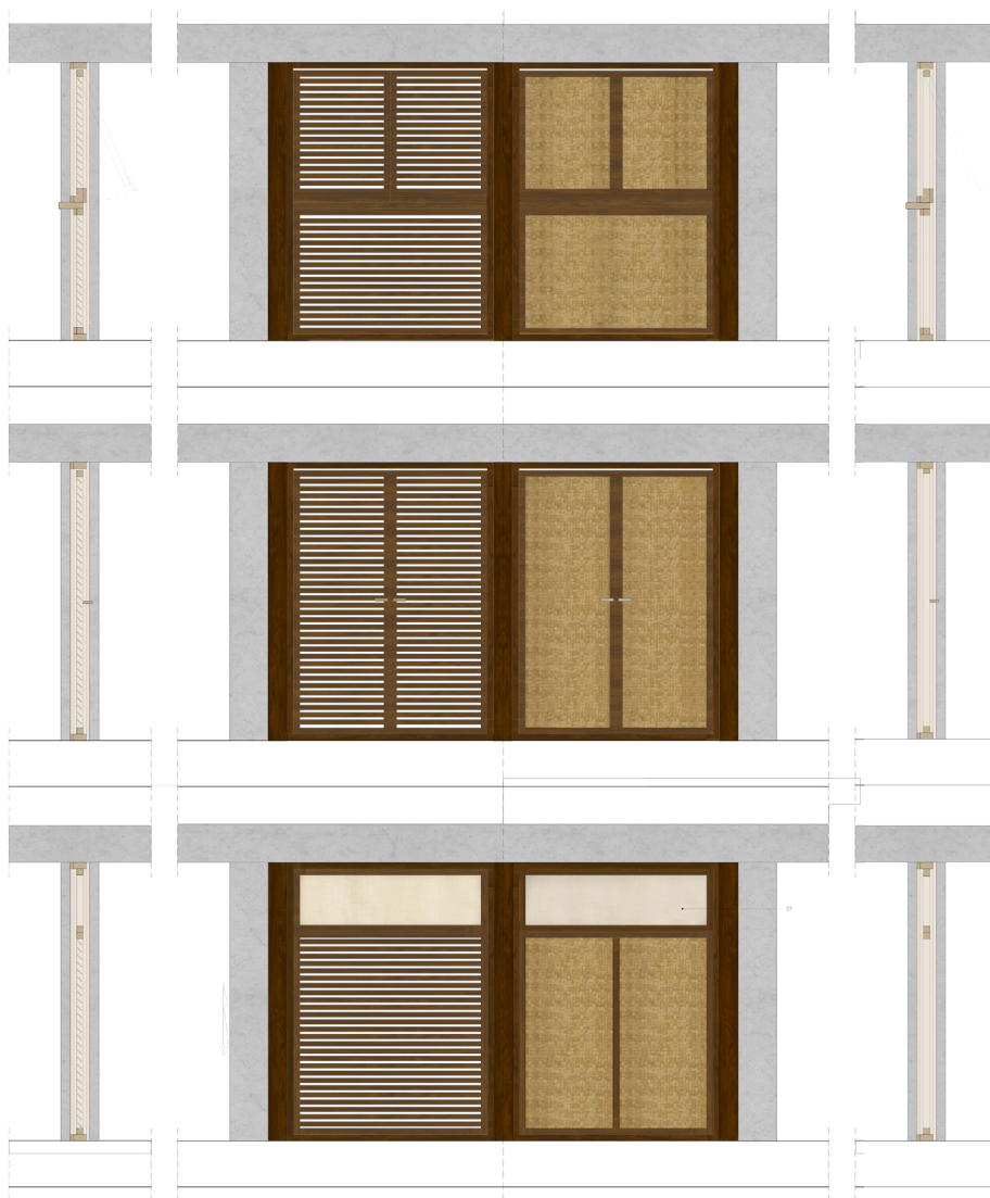
Fig. 44 – Lightweight external wall panels. The frames are in coconut palm wood, while the panels could be either in coconut palm wood slats or in woven bamboo mats. From the top: window panel; door panel; fixed panel, mainly used as the bathrooms external wall.
